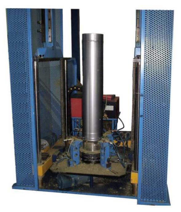
The machine is built for the assembly of tubes with double walls with cavity insulation and selfmaintenance system between the two inner and outer diameter with a minimum of 80 mm to 300 mm max interior. It is composed of a spindle to block the expansion of tire inner tube, the automatic welding of Pins, the subsequent insertion of the insulator (shells) in manual mode and the coupling of the mechanical outer and inner tube.
