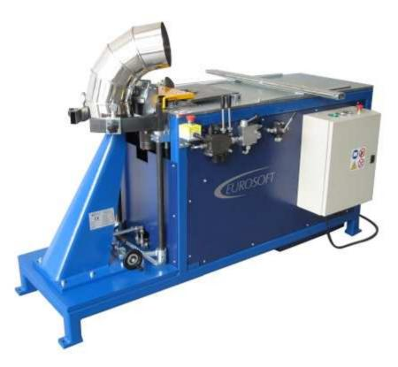
Hydraulic machine for the manufacture of elbows, reductions and covers composed of two separate workstations:
