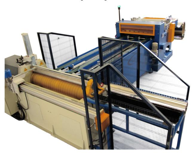
Rolling line for the building of round and oval tubes. It is composed of the following modules:
