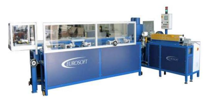
Machine for tubes production of aluminum and stainless steel crimped.
